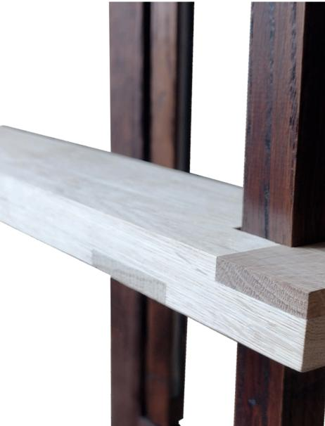
By gluing two pieces of wood with the grain perpendicular to each other, we not only enhance the beauty of the Shelf but also its strength.
